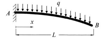
Figure 1: Sandwich cantilever beam with uniformly distributed load.
